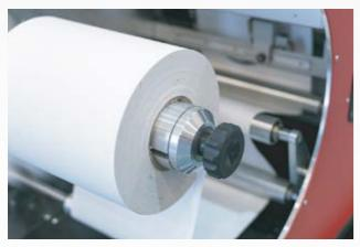
• Feeder up to 300 mm for blank or pre-diecuted rolls.
