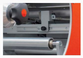
• Light sensor for reading pre-diecuted label rolls.
